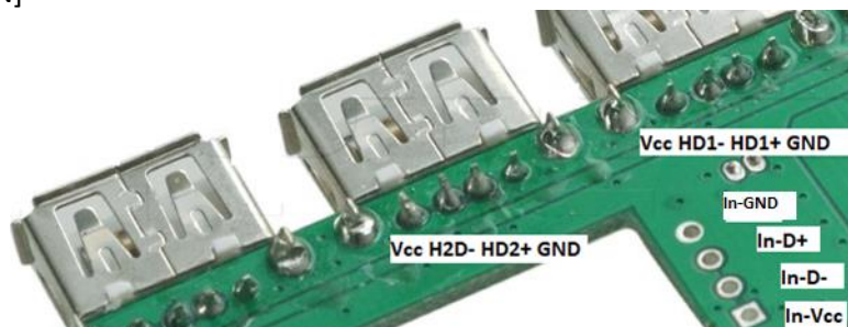
Figura 4 Pinout HUB USB
